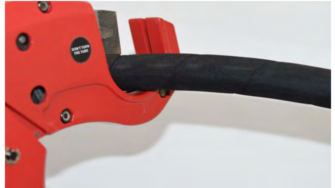
2 Cut the end of the hose using the manual cutter
