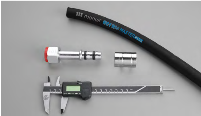
1 Check the dimensions of the components
